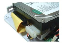
12. Use the supplied screws to secure both sides of the drive
